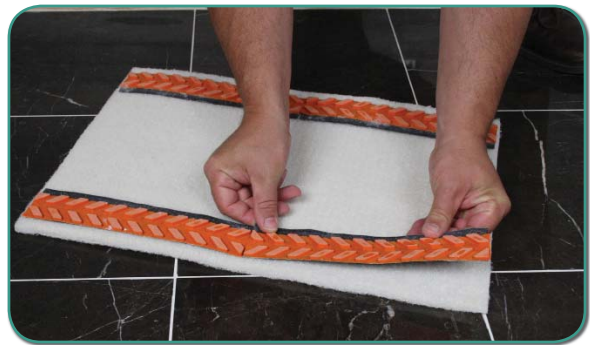
FIGURE 1-A: THE POSITION 1/2" FROM THE EDGES OF THE WHITE PAD DRIVER IS SO THAT THE DIAMOND STRIPS ARE DIRECTLY UNDER THE GRIP FACE. IF NEEDING TO GET CLOSE TO A WALL - MOVE 2 STRIP TO THE OUTER MOST EDGE AND THE OTHER DIAMONDS 1" FROM THE OTHER EDGE.
