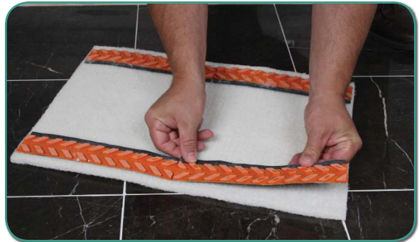
FIGURE 3-A: THE POSITION 1/2” FROM THE EDGES OF THE WHITE PAD DRIVER IS SO THAT THE DIAMOND STRIPS ARE DIRECTLY UNDER THE GRIP FACE. IF NEEDING TO GET CLOSE TO A WALL - MOVE 2 STRIP TO THE OUTER MOST EDGE AND THE OTHER DIAMONDS 1” FROM THE OTHER EDGE.
